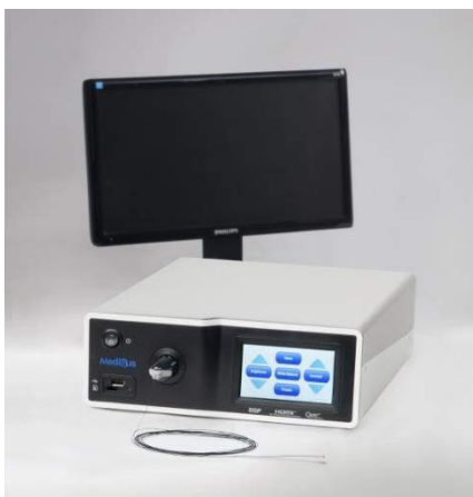
FIGURE 2-1: MICRO SCOUTCAM™ DSP SYSTEM OVERVIEW
